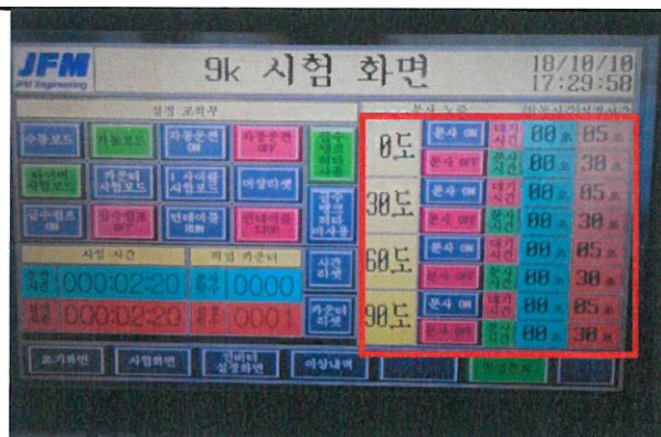
Fig. 18) Photo of the test condition (Exposure time - 30 s per position)
